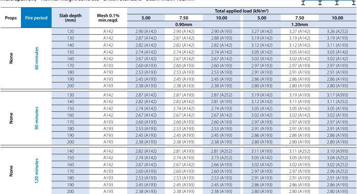
Spans are based on beam centres, with a 152mm flange width and a minimum end bearing of 50mm.
