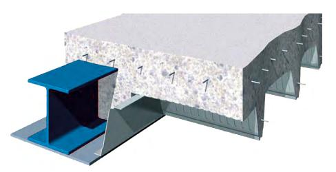
Slimflor® fabricated beam (SFB), which is a Universal Column section with a wide flange plate welded to its underside.
