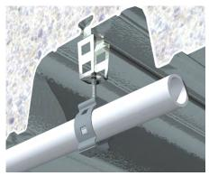
GTD-clip hangar fixings are cold-formed thin steel hangers with circular openings in the soffit to take metric bolts, threaded rods or further pipe clamp hangers. The system is installed after the composite slab has been poured and the concrete is sufficiently hardened.
