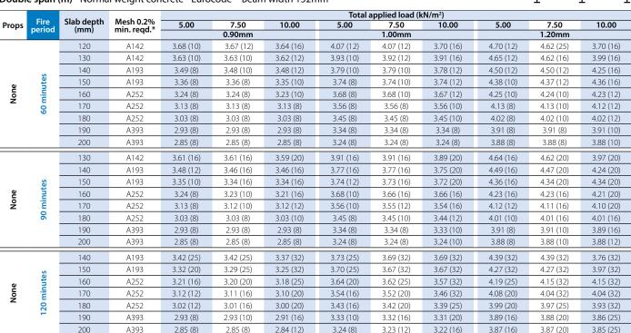
Spans are based on beam centres, with a 152mm flange width and a minimum end bearing of 50mm.
