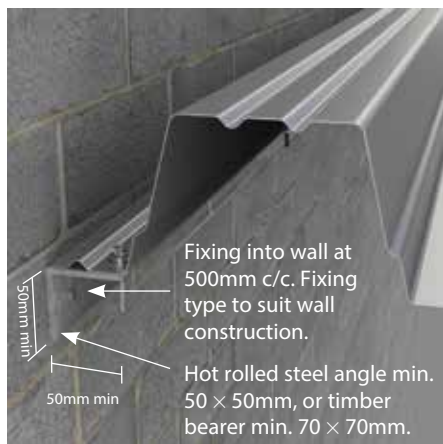
Deck verge detail. Wall abutment
